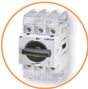
Terminal covers provide protection against accidental contact and phase separation of the switch, while perforation allows temperature monitoring of the contacts without removing the covers
