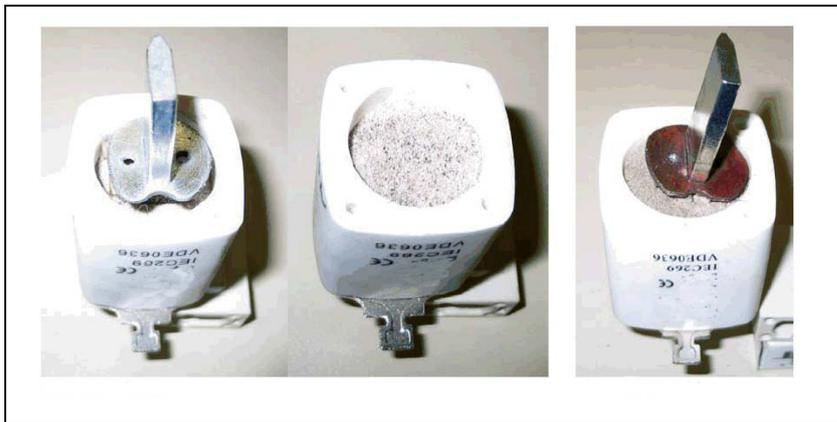
**Fig. 4** To low level of the quartz sand in arched chamber for the fuse imported from Far East.
