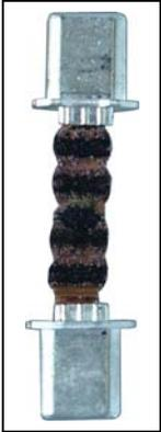
Fig. 3 Burned fuse element
