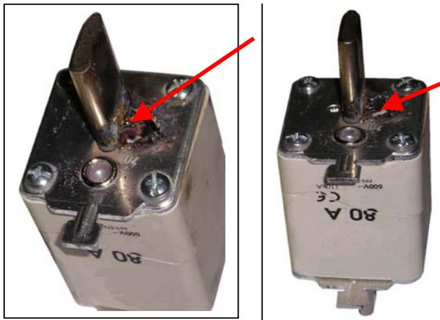
**Fig. 5** Get out of the voltaic arc, because of the to small level of the quarto sand.
