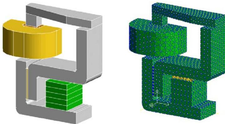
Figure 2: Geometry of magnetic circuit for the calculation of electromagnetic field
